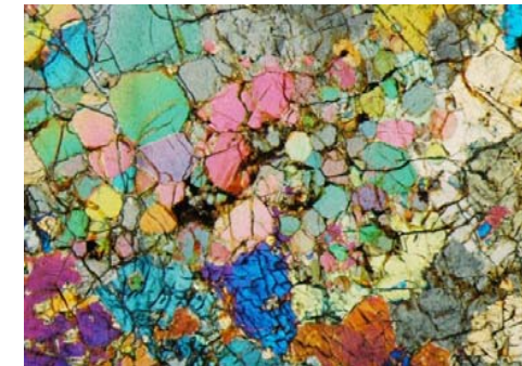
Figure 9. Dhofar 700. Cluster of polygonal olivine (xenolith?) with partial poikilitic margin (right margin) of olivine chadacrysts and orthopyroxene host. Base width = 9 mm; crossed polarizers.
